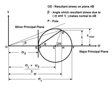
3. Shear stress is generally taken as positive if it causes CCW couple at a point inside the wedge ABC.
