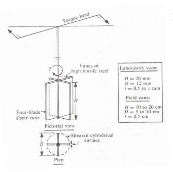
Shear failure occurs over the surface and the ends of a cylinder having a diameter D, equal to the diameter of the vane.
