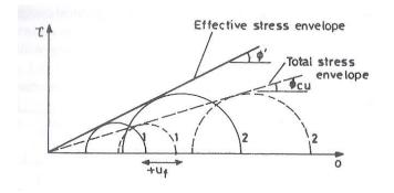
In normally consolidated clays there is a tendency towards volume decrease under undrained conditions during shear (that is, for pore water to escape). If this volume change is not allowed to occur, positive pore water pressures develop. Consequently, effective stress Mohr circles lie to the left of total stress circles (i.e. effective stress < total stress). **Both** effective stress and total stress failure envelopes the normally for
