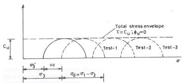
In this test, cell pressure during the consolidation phase is applied without allowing drainage. Then keeping cell pressure constant, deviator stress is increased to failure without drainage. Thus, the drainage valve is closed throughout the test. This is a total stress test and does not usually intend measuring the pore pressures. It is
