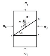
The critical stress values generally occur on planes normal to the intermediate plane. Consider a plane AB of unit width perpendicular to the plane of the paper, inclined at  $\theta$  to the major principal plane.
